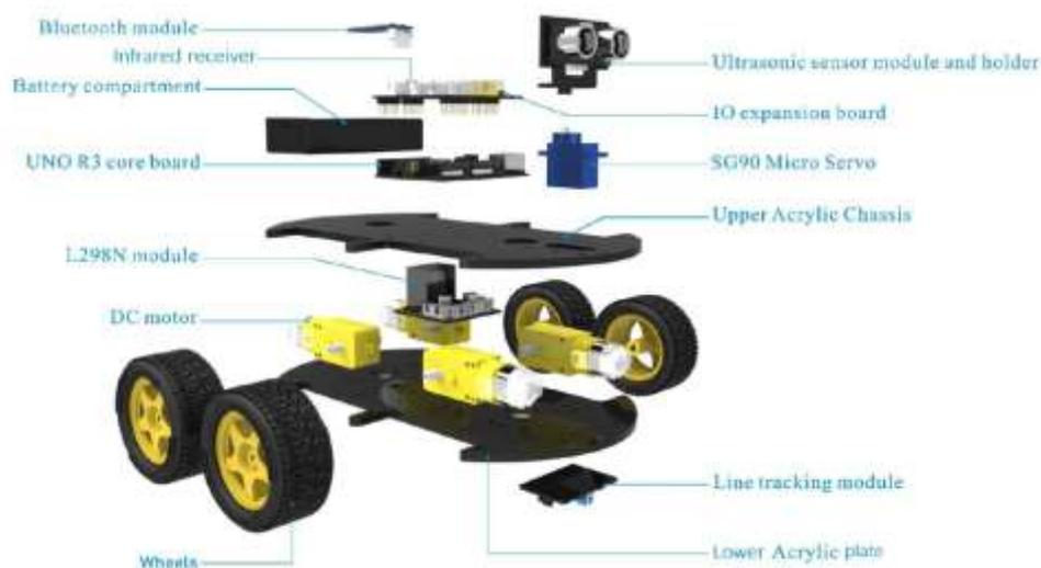
Figure 3.4: Exploded assembly of the system
