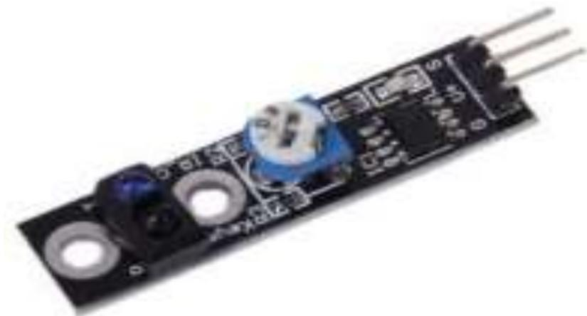
Figure 4.1.2: Line tracking sensor assembly
