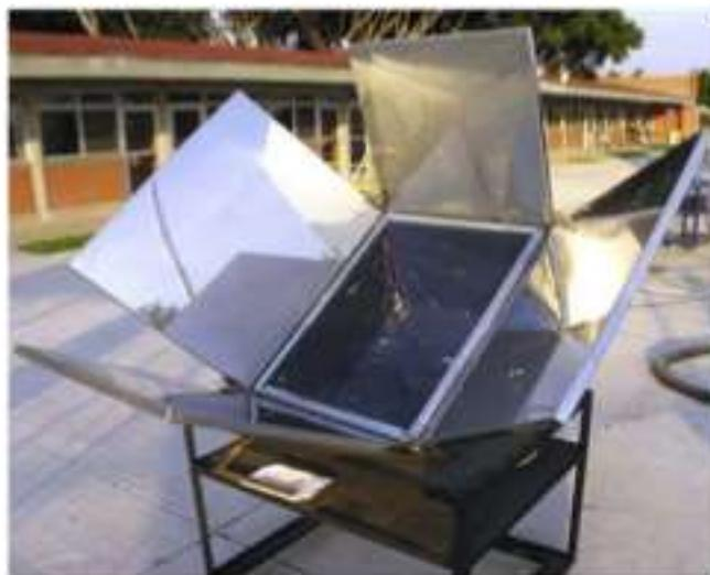
Figure 2.1: A photograph of the constructed oven prototype.
