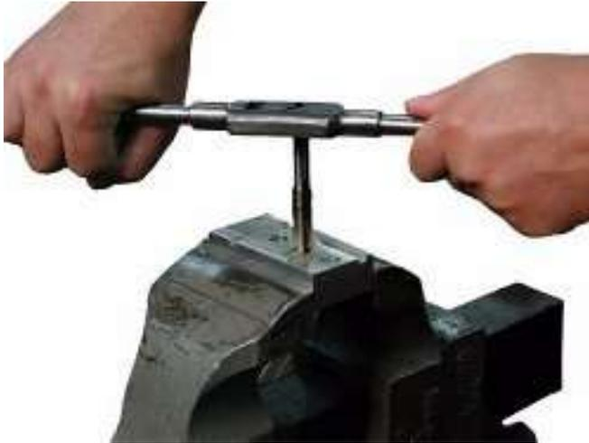
Figure 10: Manual tapping experimental setup
