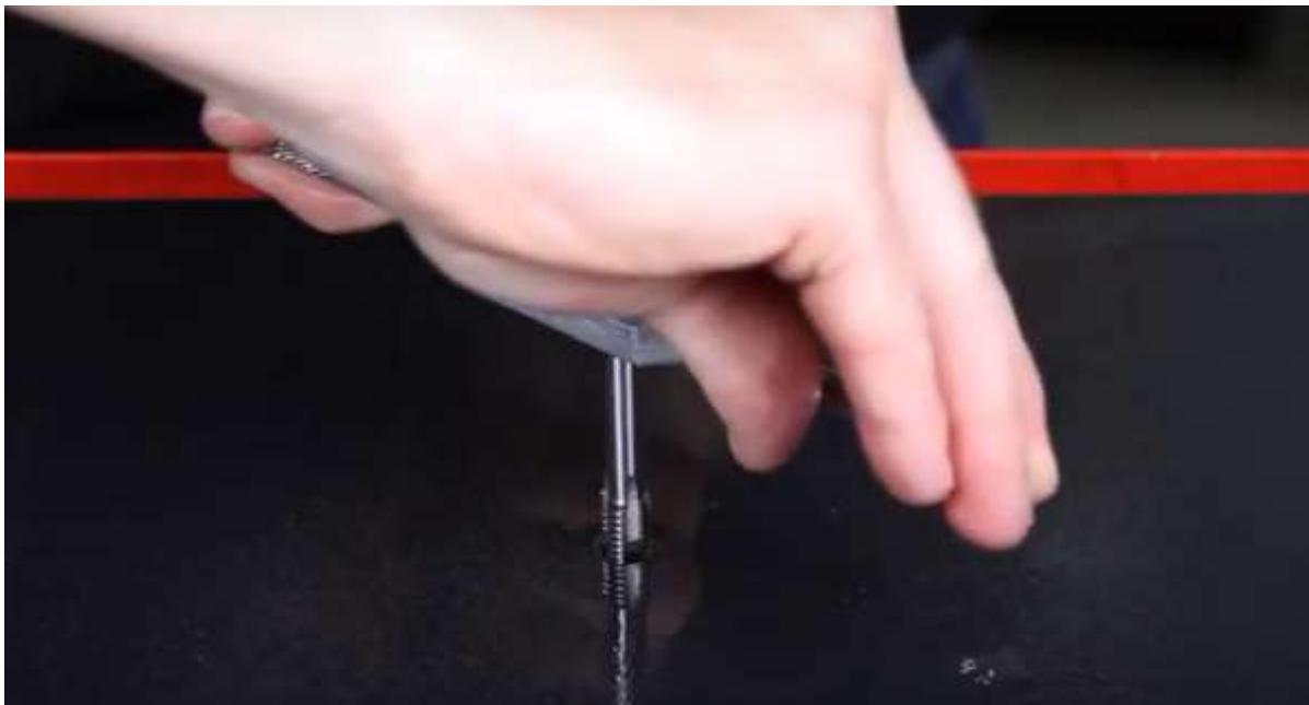
Figure 11: Manual tapping process
