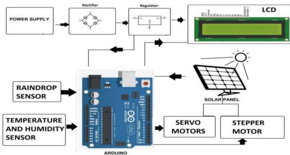
Figure 1 Initial flow diagram of solar panel with weather sensor kit
