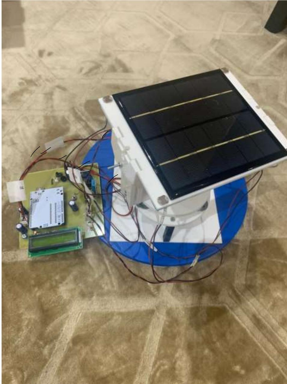
Figure 13 Demonstration of solar tracker
