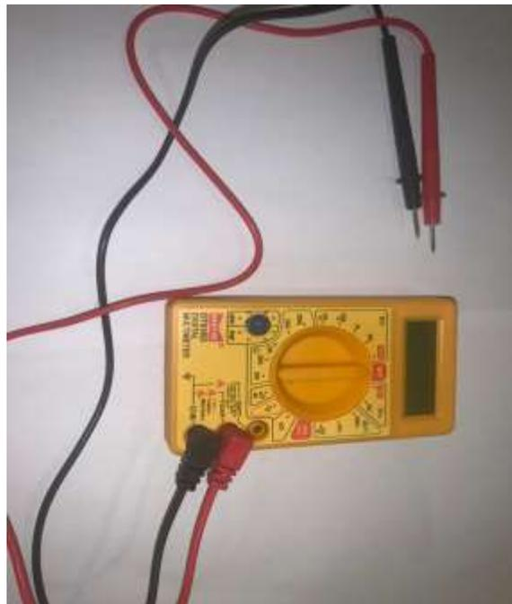
Figure 8 Digital multimeter
