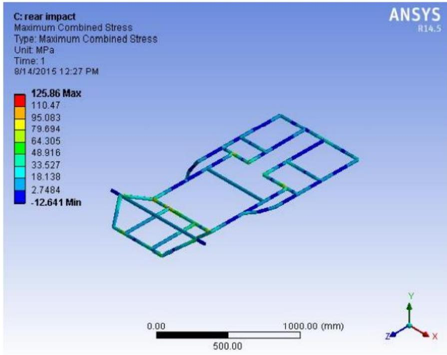
Figure 9: Rear Impact Test of chassis in Ansys workbench
