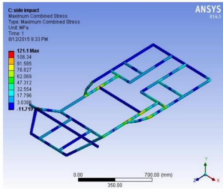
Figure 10: Side impact test of chassis in Ansys workbench
