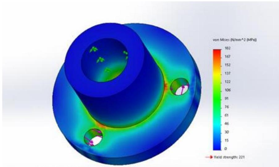
Figure 11: Analysis of wheel hub in Ansys workbench
