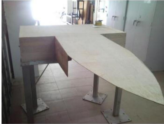
Figure 3: Plywood molding of Go-Kart (Hui, 2011)
