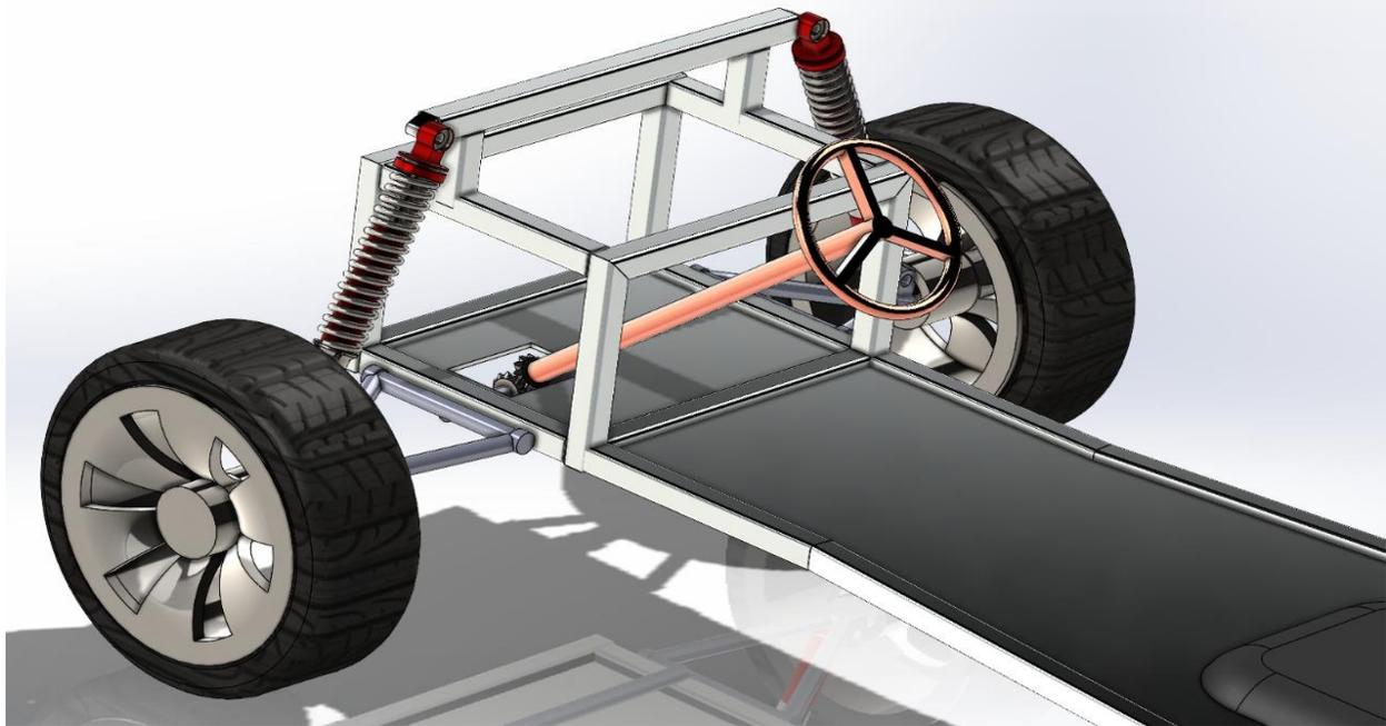
Figure 6: Steering mechanism of Go-Kart
