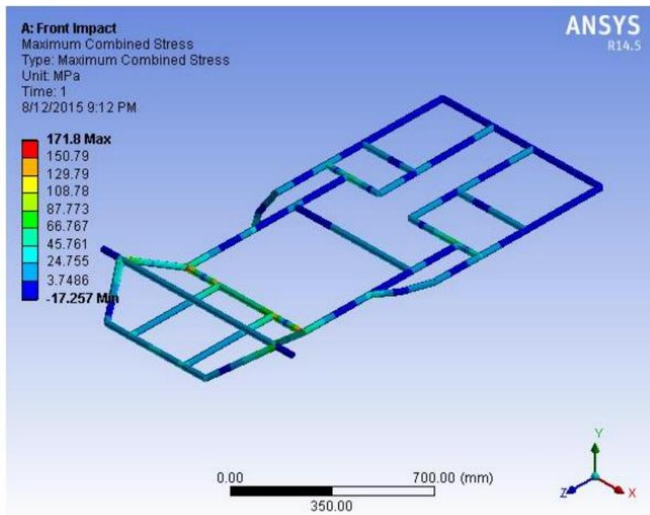
Figure 8: Front Impact test of chassis in Ansys work Bench
