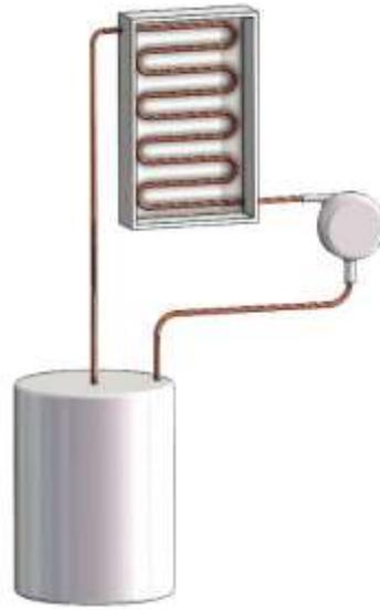
Figure 10 Solar water heater design
