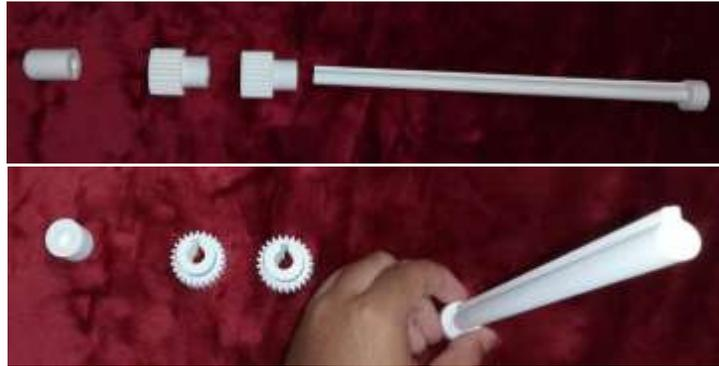
7- Insert into the hole on the side of the base, and pair (fit) each pinion to a rack gear
