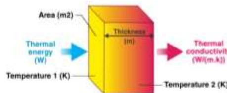
Figure 12 Heat Transfer Diagram
