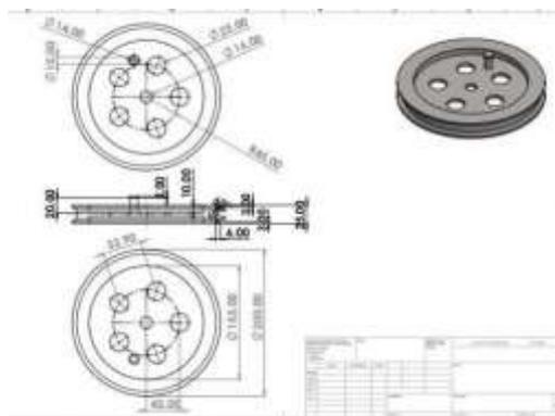
Figure 11 1st Pulley
