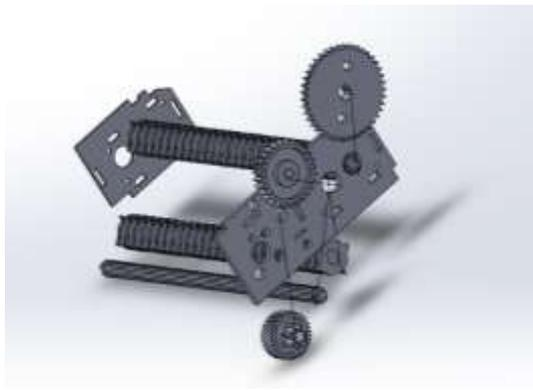
*Figure 10: Exploded Assembly of the system*
