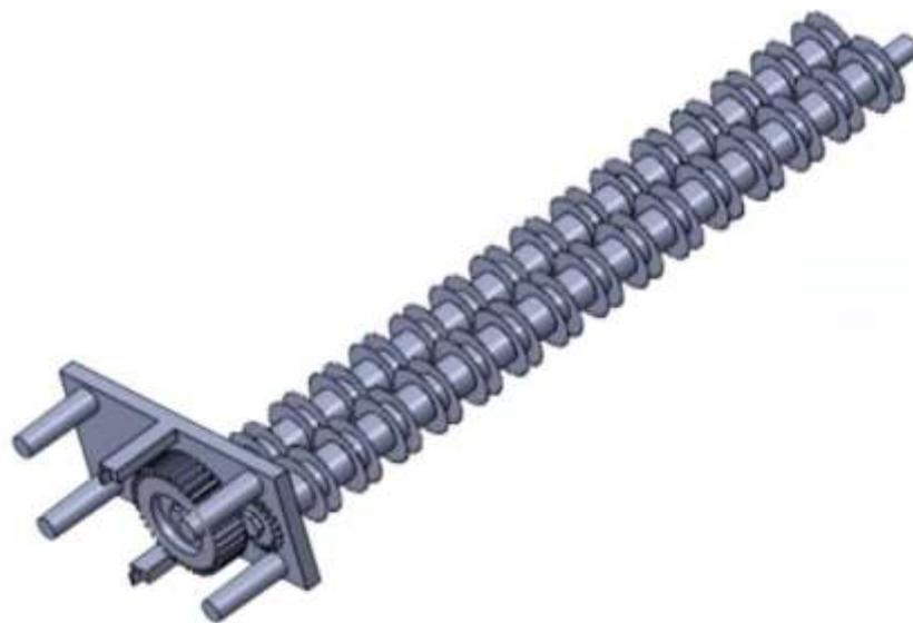
*Figure 1: Designing cutting blades and gears in SolidWorks*
