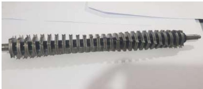
*Figure 9 :The used AISI 304 stainless-steel shaft and blades*
