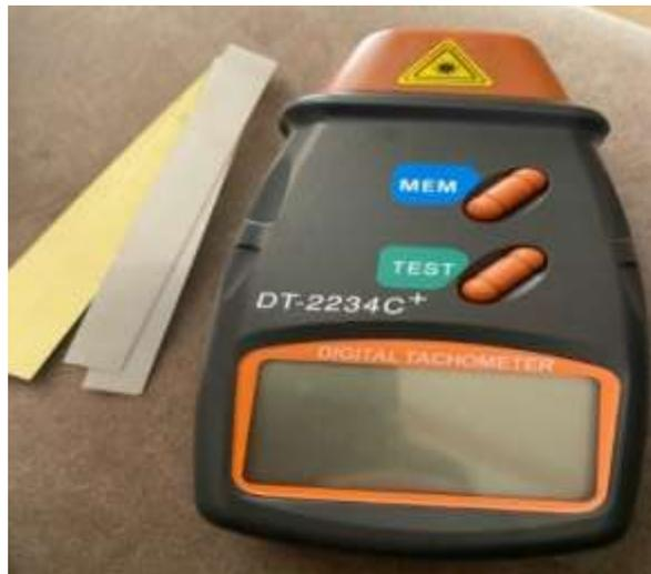
*Figure 17: Tachometer Device with Stickers*
