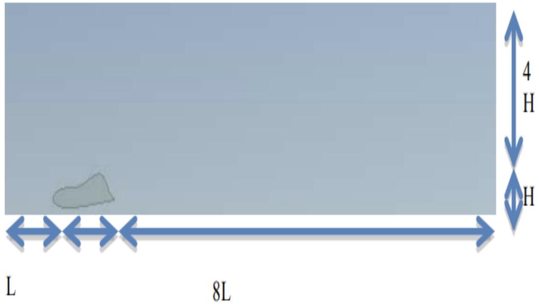
Figure #2.1 Computational Domain for CFD Simulation Setup (Front View)
