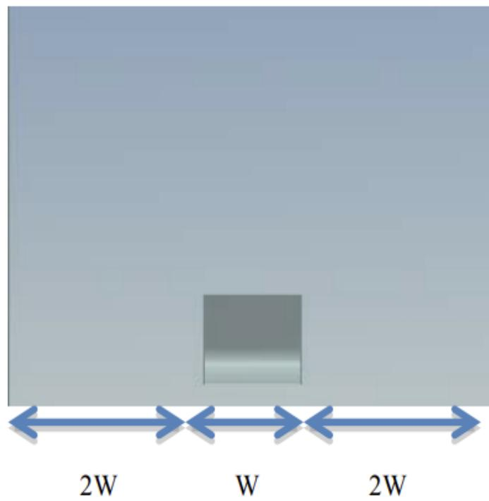
Figure #2.2 Computational Domain for CFD Simulation Setup (Side View)
