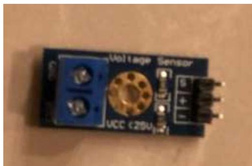
Figure#3.4(c): Voltage sensor
