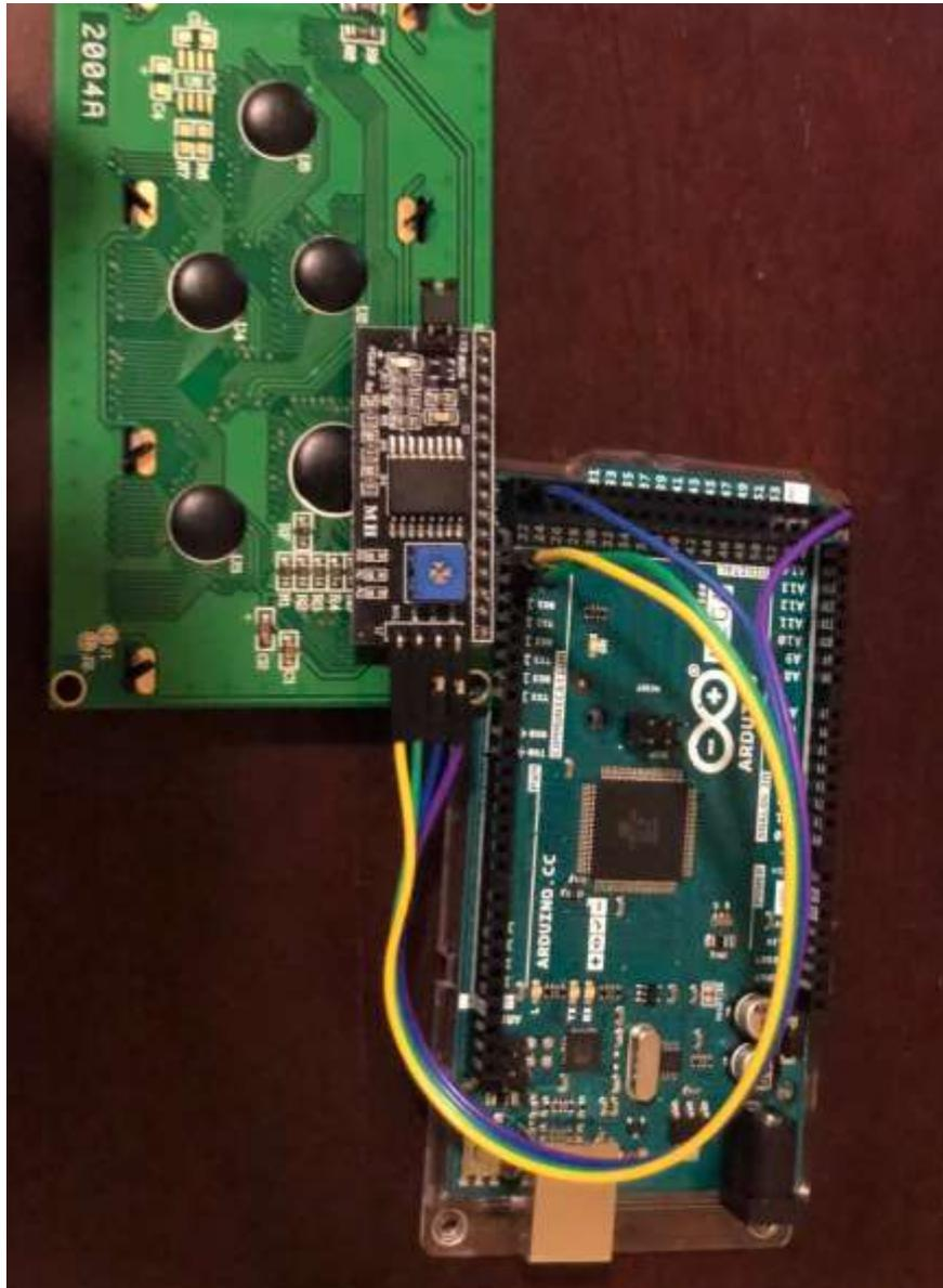
**Figure# 4.2: Arduino connected to LCD**
