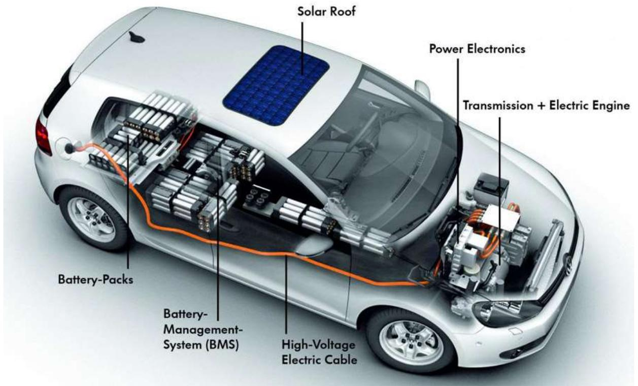
Figure#3.5: Idea of engine of solar-electric car
