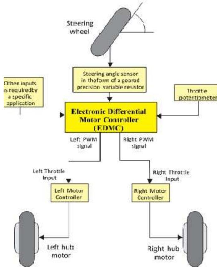
**Figure 3: Electronic differential system for electric vehicle**
