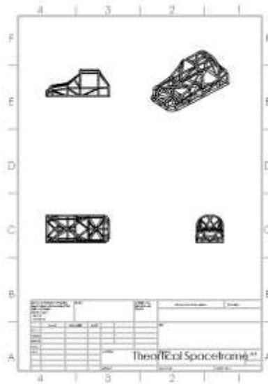
Figure 3.3.2: Simple Spaceframe Chassis Drawings
