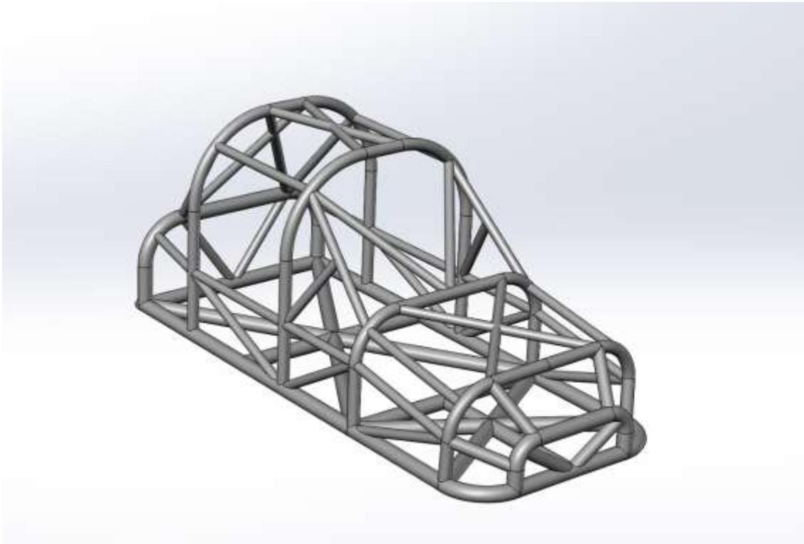
Figure 3.3 1: Simple Spaceframe Chassis model
