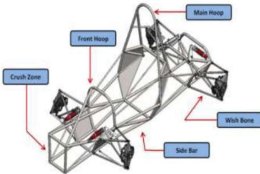
**Figure 2.2:** An example of space frame race car chassis structure based on Formula SAE specification.
