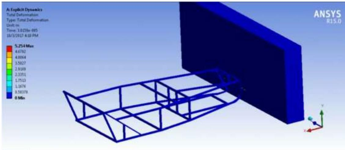
Figure 3.3.3: Total Deformation
