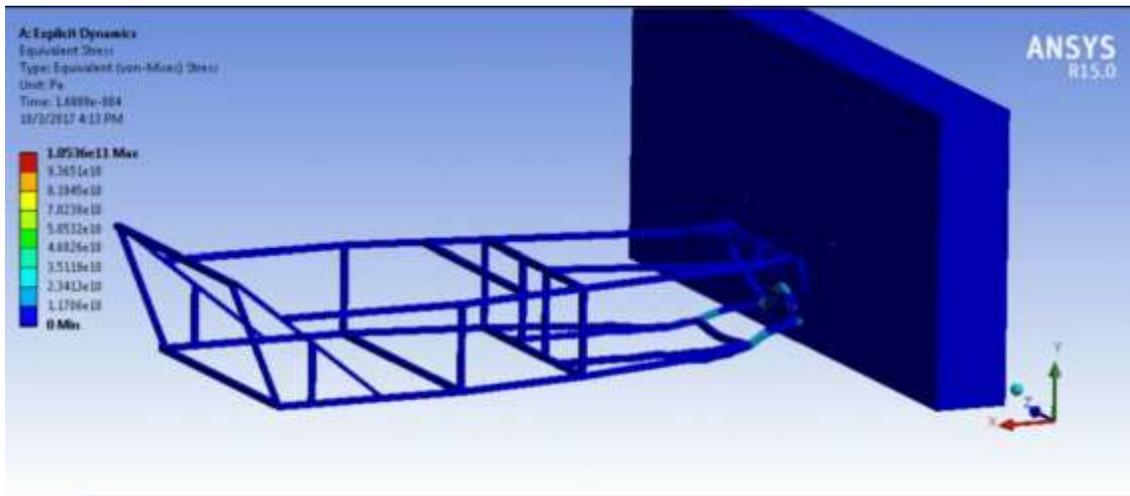
Figure 3.3.4: Equivalent Stress
